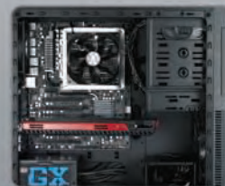
Support long VGA card with removable HDD Cage (ATI HD6990)
