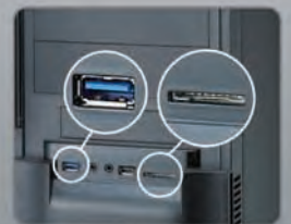
Support USB 3.0 and High speed SDHC card reader
